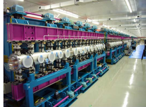
In-vacuum type undulator Period 18mm
