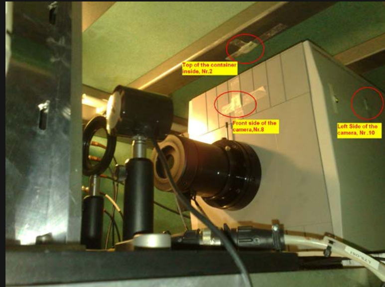
Hence, we housed the Streak Camera in a shielded (neutron and gamma) container. The monitoring dosimeter locations are indicated.
