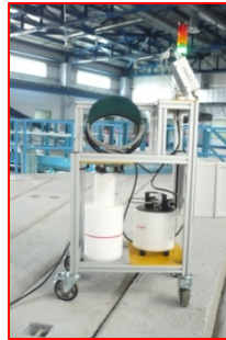
FHT 192 Gamma Ionization Chambers, Energy Range 30 keV to 7 MeV( \pm 30\% ), Dose Range 10 \mu R/h to 100 R/h
