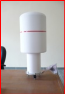
FHT 192 Gamma Ionization Chambers, Energy Range 30 keV to 7 MeV( \pm 30\% ), Dose Range 10 \mu R/h to 100 R/h
