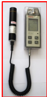
2 FH 40 G portable digital gamma survey meter, Energy Range 30KeV to 4.4MeV
