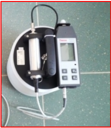
2 Portable FHT 762 Wendi-2 Wide-Energy Neutron Detector, Energy Range 25meV to 5GeV
