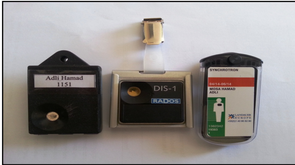
Fig.1: different types of personal dosimeters used at SESAME
